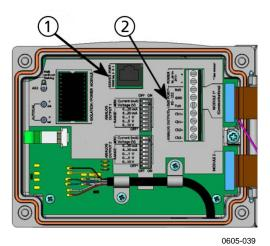
Figure 51 Service Port Connector and User Port Terminal on Motherboard
