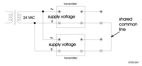
Figure 21 Connections to 24 VAC Power Supply
