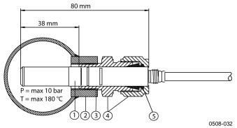
Figure 94 Swagelok Installation Kit for RH-probe
