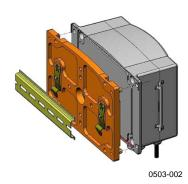
Figure 10 Mounting with the DIN Rail Installation Kit
