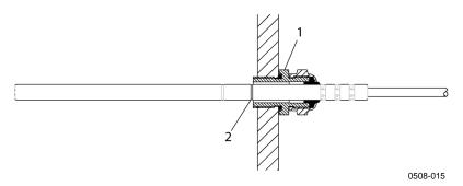
Figure 98 Vapor Tight Installation
