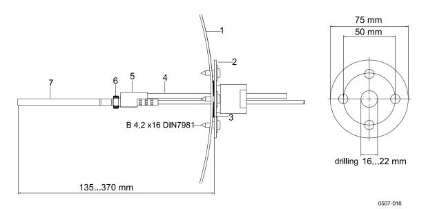
Figure 93 Duct Mounting Installation Kit for T-Probe
