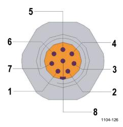
Figure 42 Pinout of the Optional 8-Pin Connector
