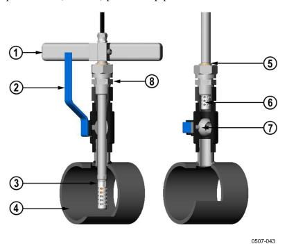
Figure 102 Installing the HMT338 Probe Through a Ball Valve
