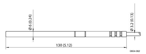
Figure 91 Optional Temperature Probe Dimensions
