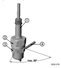
Figure 30 Tightening the Clasp Nut
