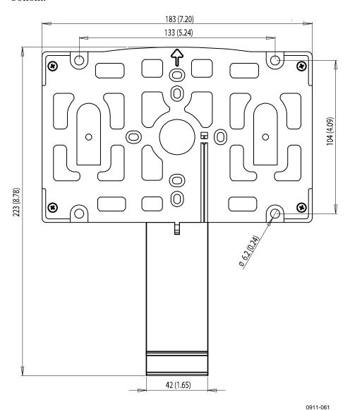
Figure 9 Dimensions of the Probe Holder Plate (mm/inch)
