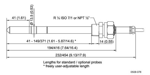
Figure 90 HMT338 Probe Dimensions
