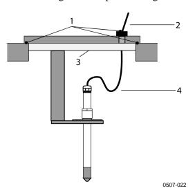
Figure 24 Vertical Mounting of Probe
