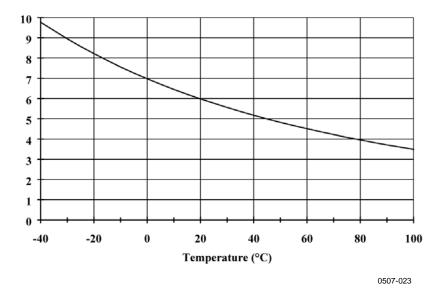
Figure 22 Measurement Error at 100 %RH
