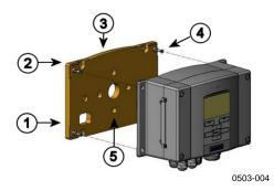
Figure 7 Mounting with Wall Mounting Kit
