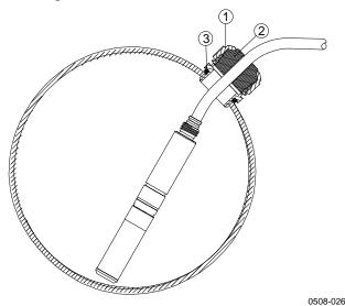
Figure 96 Cable Installation with Cable Gland
