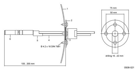
Figure 92 Duct Mounting Installation Kit
