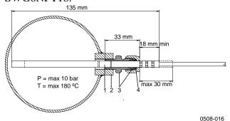
Figure 95 Swagelok Installation Kit for T-Probe
