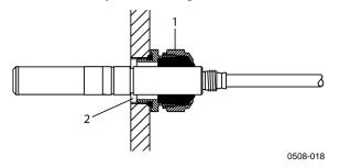
Figure 97 Probe Installation with Cable Gland
