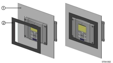
Figure 16 Panel Mounting Frame
