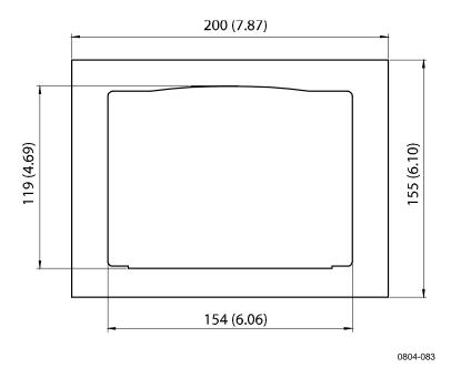
Figure 17 Panel Mounting Dimensions (mm/inch)
