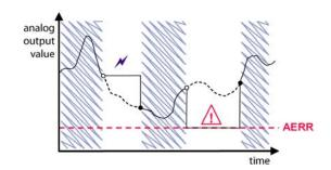
Relay is released when the output values are frozen, the adjustment mode is activated, or an instrument failure is detected
