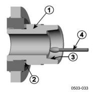
Figure 27 Cleaning of Tightening Cone
