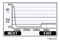
Figure 47 Alarm Limits Shown on Graph Screen
