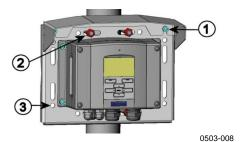
Figure 15 Mounting the Rain Shield with the Installation Kit
