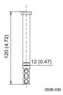
Figure 84 HMT331 Fixed Probe Dimensions
