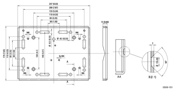
Figure 14 Dimensions of the Metal Mounting Plate (mm/inch)
