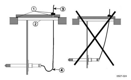
Figure 23 Horizontal Mounting of Probe
