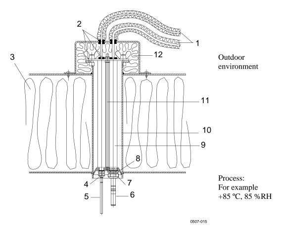
Figure 101 Example of Installation through Roof
