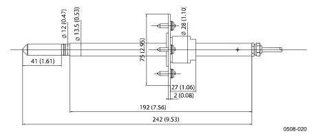
Figure 88 HMT335 Probe Dimensions
