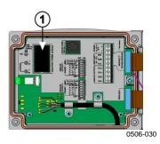
Figure 32 Galvanic Isolation Module
