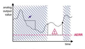
Relay is released in case of a measurement failure only.
