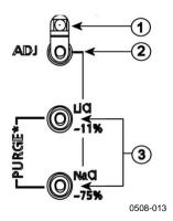
Figure 77 Adjustment and Purge Buttons
