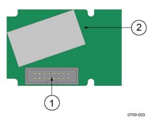
Figure 39 LAN Interface Module
