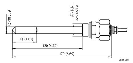
Figure 87 HMT334 Probe Dimensions
