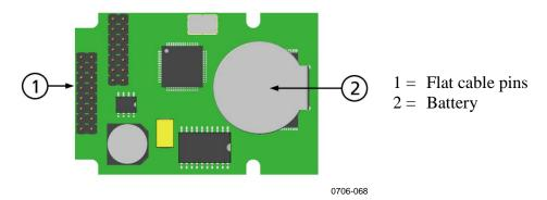
Figure 41 Data Logger Module
