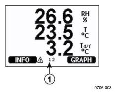
Figure 65 Relay Indicators on Display
