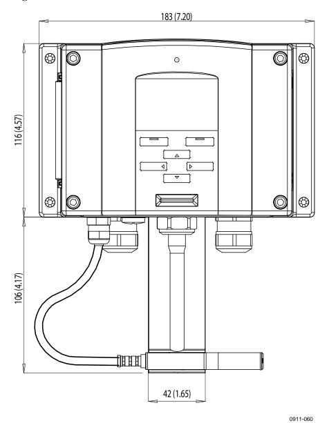
Figure 85 HMT331 Short Cable Probe Dimensions
