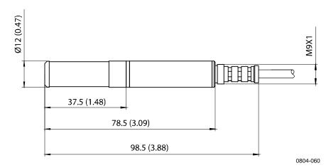
Figure 86 HMT333 Probe Dimensions
