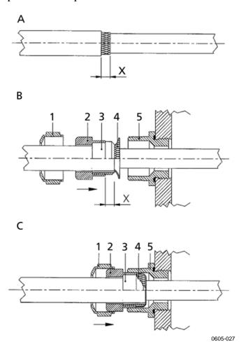
Figure 19 Grounding the Screen of Electrical Cable
