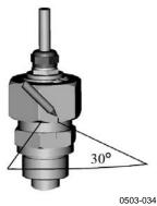
Figure 26 Tightening the Nut
