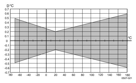
Figure 80 Accuracy over Temperature Range
