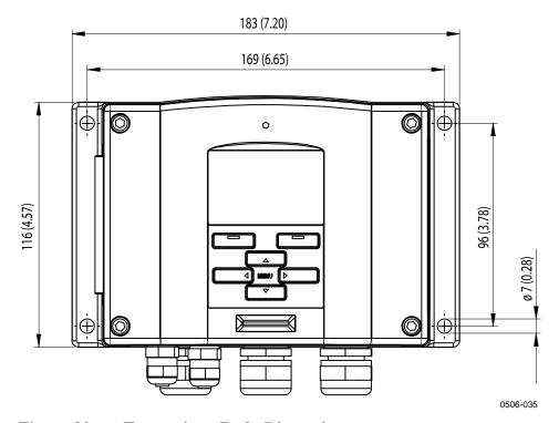
Figure 82 Transmitter Body Dimensions
