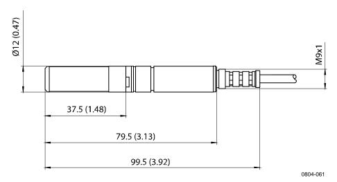
Figure 89 HMT337 Probe Dimensions
