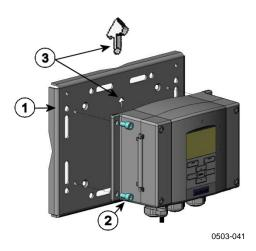
Figure 13 Mounting with Metal Wall Mounting Plate
