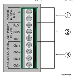
Figure 20 Screw Terminal Block on Motherboard
