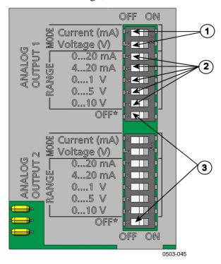
Figure 62 Current/Voltage Switches of Output Modules
