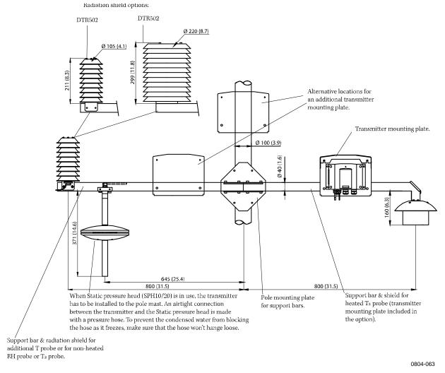
Figure 103 Meteorological Installation Kit for Outdoor Installation
