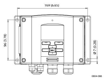
Figure 6 Standard Mounting
