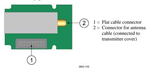
Figure 40 WLAN Interface Module
