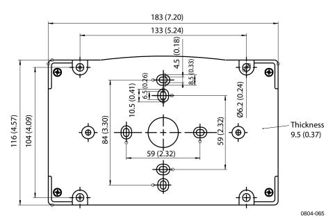
Figure 8 Dimensions of the Plastic Mounting Plate (mm/inch)
